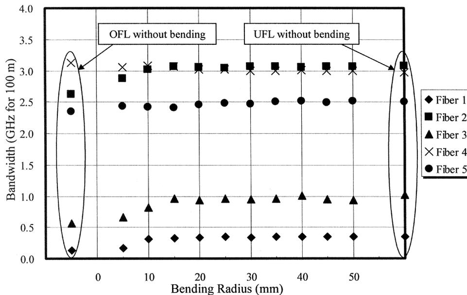
Fig. 10. Bandwidths of the GI POFs under UFL before and after bending compared with the one under OFL without bending.
