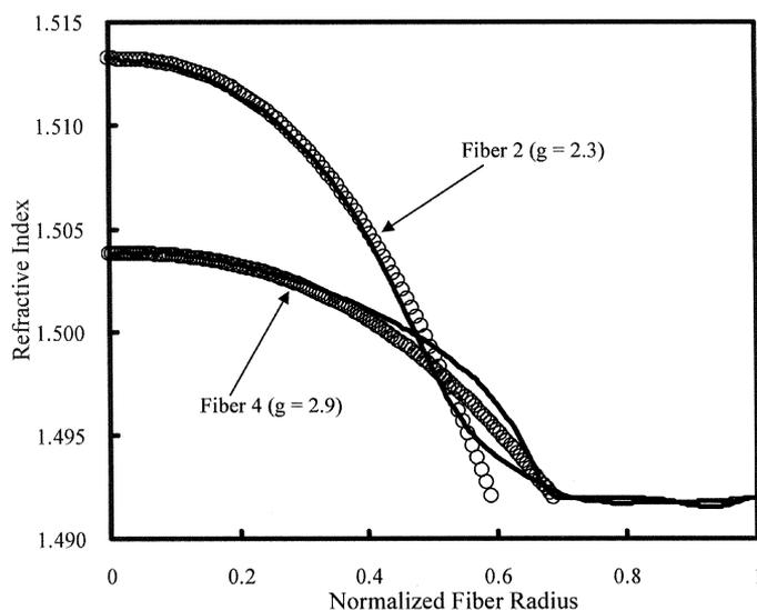
Fig. 6. Measured (solid line) refractive-index profiles of fibers 2 and 4 compared with optimum one (open circle:  $g = 2.4$ ).
