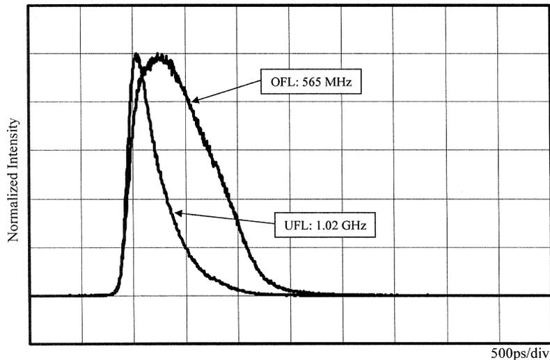
Fig. 9. Output pulse waveforms through 100-m fiber 3 under UFL and OFL.
