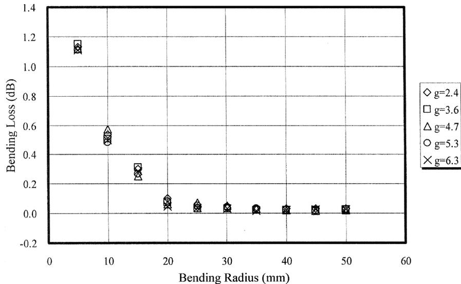
Fig. 13. Bending losses of the GI POFs with different index profiles.
