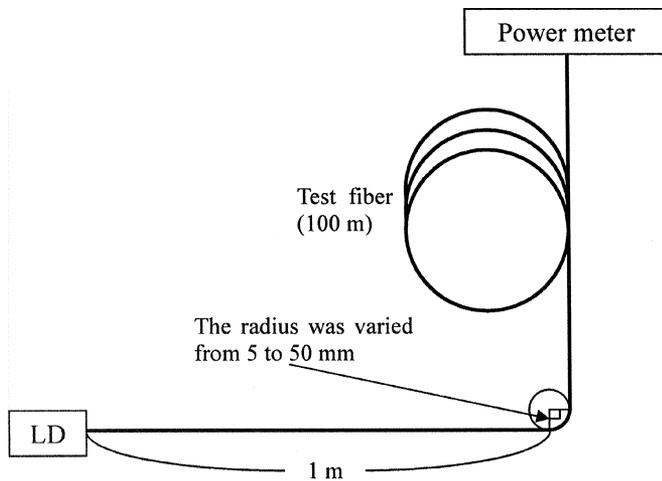
Fig. 1. Schematic diagram of the bending condition.
