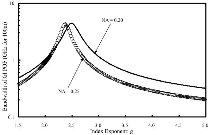
Fig. 3. Relation between index exponent  $g$  and bandwidth of 100-m PMMA-based GI POF with different NAs: 0.20 and 0.25.
