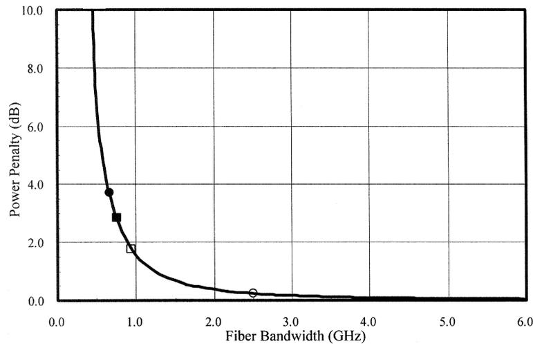
Fig. 15. Calculated relation (solid line) between the fiber bandwidth and the power penalty for 1.25-Gb/s transmission (fiber length = 100 m). o: The link performance of fiber 5 without bending. ●: The link performance of fiber 5 under the 90° bending with 10-mm radius. □: The link performance of fiber 3 without bending. ■: The link performance of fiber 3 under the 90° bending with 10-mm radius.
