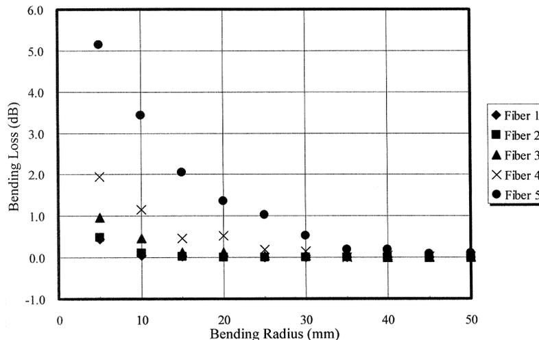
Fig. 14. Bending losses of the GI POFs with different NAs.
