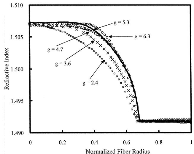
Fig. 12. Refractive-index profiles of the GI POFs with almost the same NA and core diameter.
