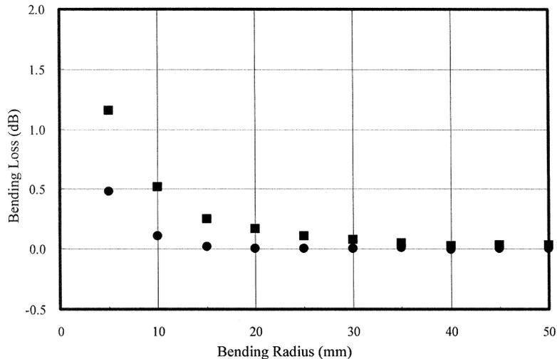
Fig. 11. Bending losses of fiber 2 under UFL and OFL.
