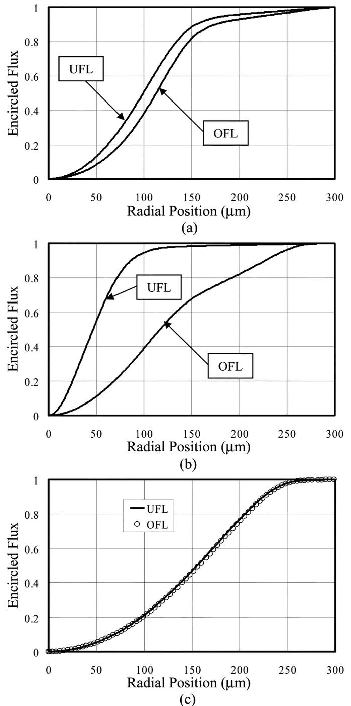
Fig. 2. EFs of the (a) 100-m and (b) 5-m GI POFs with small mode coupling (fiber 2) under UFL and OFL, compared with that of (c) a 100-m GI POF with large mode coupling.
