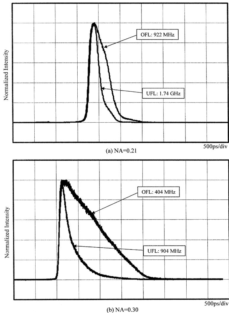
Fig. 5. Bandwidth performances of the 50-m GI POFs having almost the same index profile ( $g = 4.8$ ) and different NAs.
