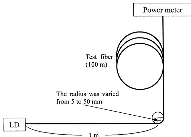
Fig. 1. Schematic diagram of the bending condition.
