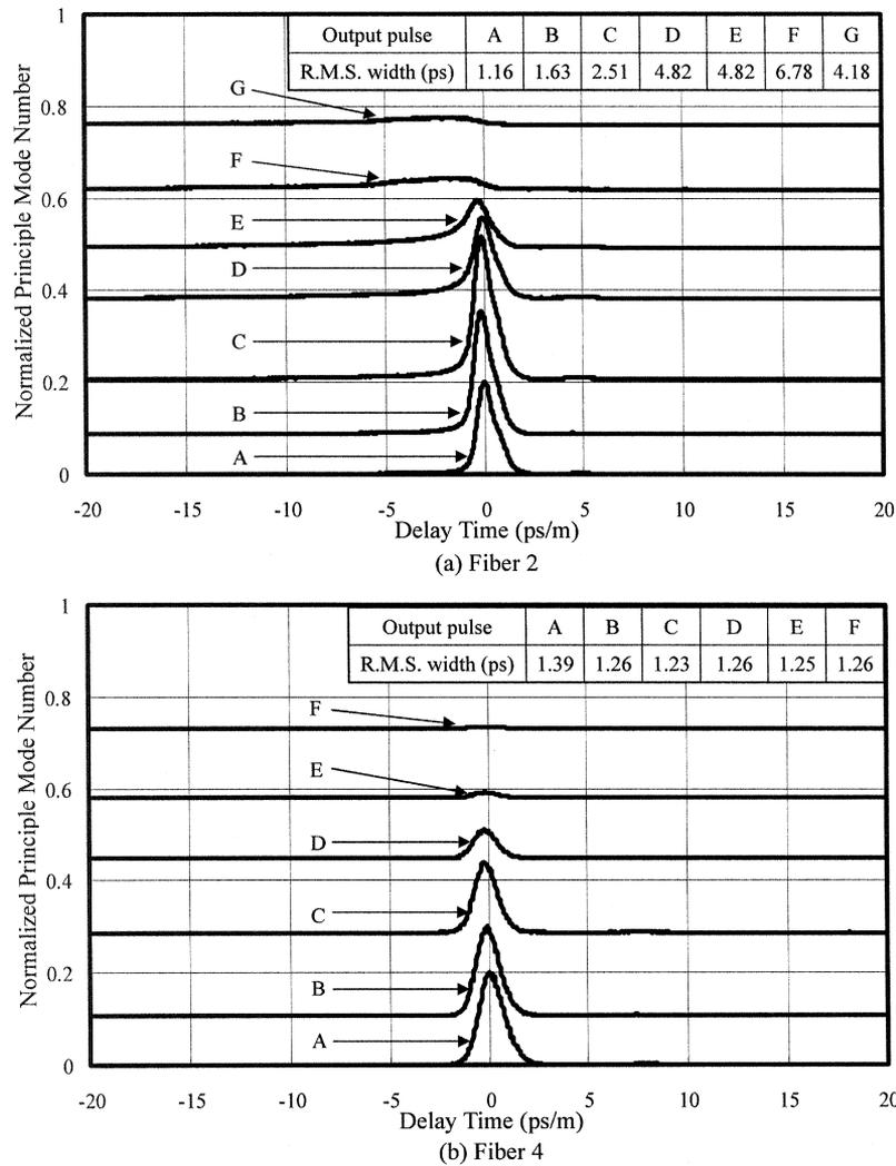
Fig. 7. Output pulse waveforms and their rms widths of differential-mode delay measurements of 100-m (a) fiber 2 and (b) fiber 4.
