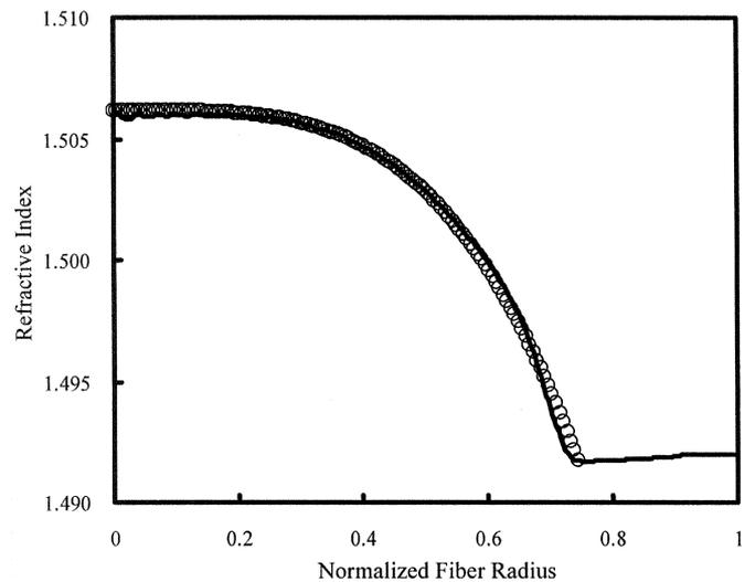
Fig. 8. Measured (solid line) and approximated (open circle:  $g = 3.7$ ) refractive-index profiles of fiber 3.
