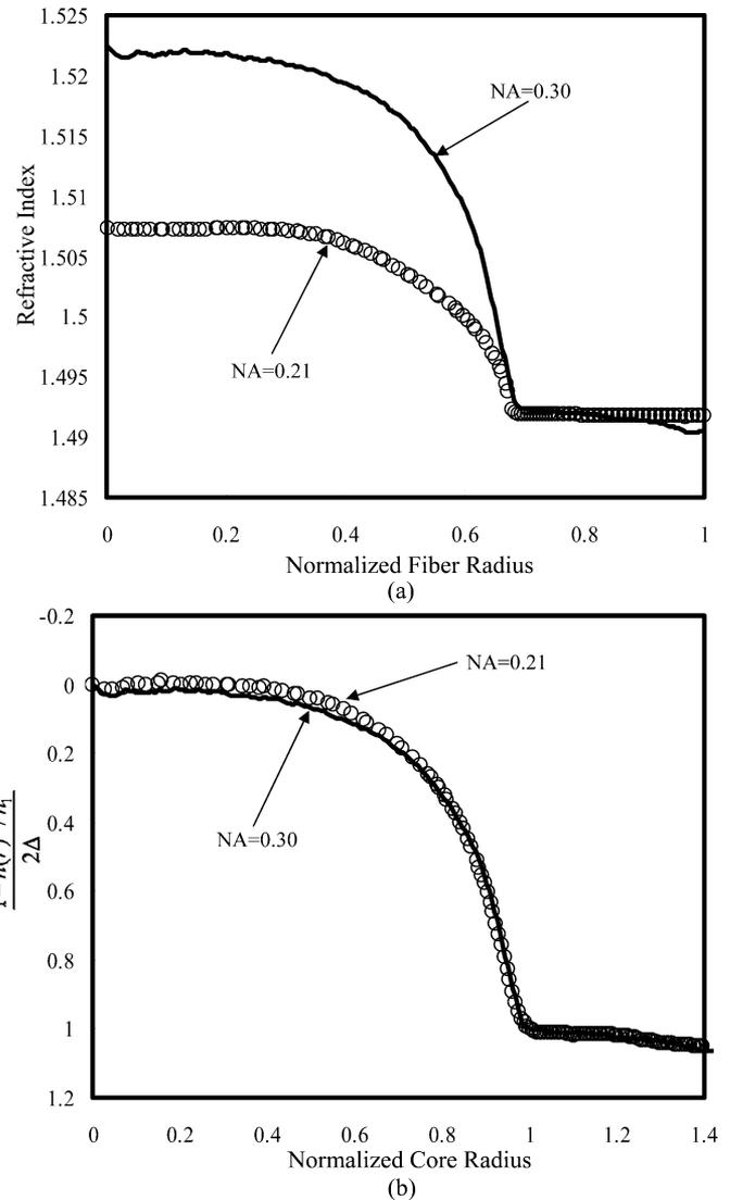
Fig. 4. (a) Measured refractive-index profile and (b) calculated profile function of the GI POFs having almost the same index profile ( $g = 4.8$ ) and different NAs.
