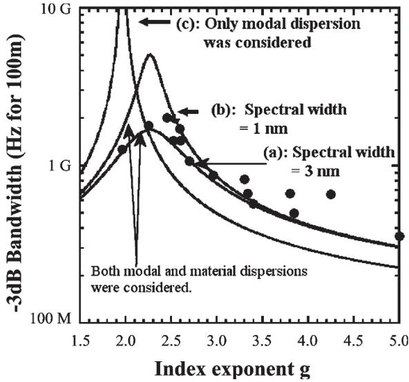
Fig. 3. Relation between the index exponent  $g$  and  $-3$ -dB bandwidth of 100-m PMMA-based GI POF at 650-nm wavelength. • Experimentally measured data (spectral width = 3 nm).
