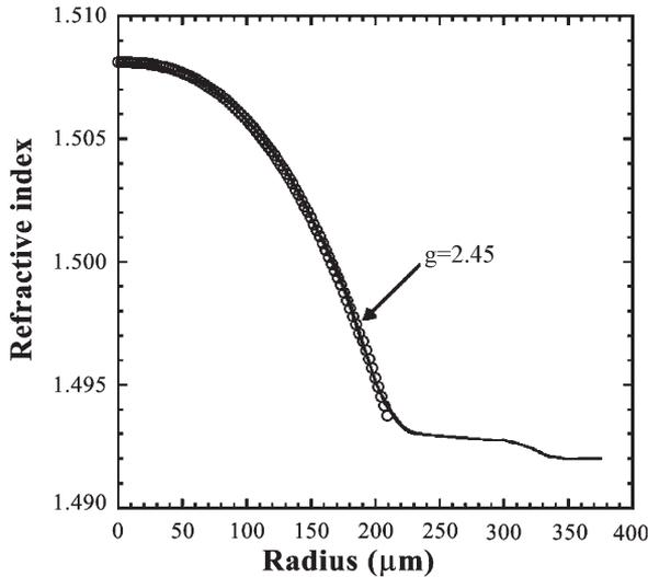
Fig. 6. Optimization of the refractive index profile of PMMA-based GI POF. Solid line: Measured index profile. Open circle: Approximated profile by a power-law form.
