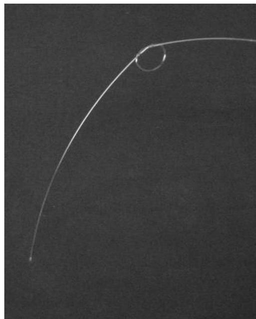
Fig. 10. Flexible GI POF. Optical signal is transmitted even if a knot is added in the GI POF.
