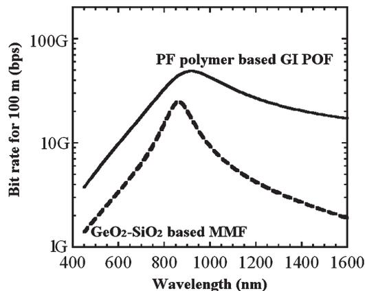
Fig. 15. Wavelength dependence of the possible bit rate in the PF GI POF link compared with that of silica-based MMF.
