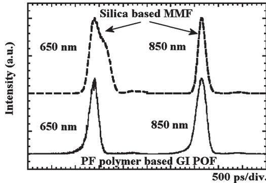
Fig. 16. Comparison of wavelength dependence of output pulse broadening from 300-m PF GI POF and silica-based MMF.
