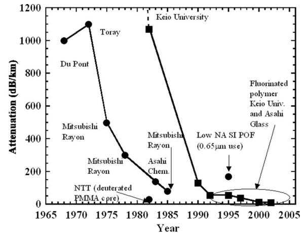
Fig. 1. Development in the attenuation of POFs. ● SI POF. ■ GI POF.
