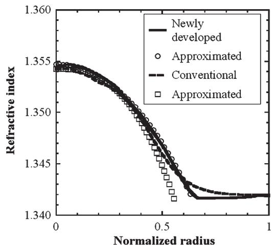
Fig. 13. Refractive index profiles of PF polymer-based GI POFs. Broken line: Measured profile formed by the conventional preparation process.  $\square$  approximated curve by power-law when  $g = 1.9$ . Solid line: Measured profile formed by newly developed process.  $\circ$  approximated curve by power-law when  $g = 2.1$ .
