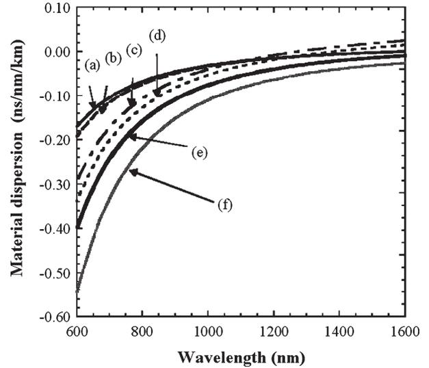
Fig. 12. Comparison of material dispersion of each polymer matrix. (a) PF homopolymer, (b) PF dopant-doped PF polymer, (c) pure silica, (d)  $\text{GeO}_2$ -doped silica, (e) PMMA, and (f) DPS-doped PMMA.
