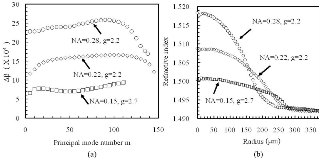
Fig. 5. (a) Fiber NA dependence of the difference between propagation constants ( $\Delta\beta$ ) of adjacent modes. (b) Refractive index profile of the GI POF used for the calculation of  $\Delta\beta$  shown in (a).
