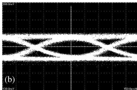
Fig. 9. (a) Bending condition of GI POF and (b) eye pattern after a 1.25-Gb/s transmission through 50-m GI POF with static bendings.
