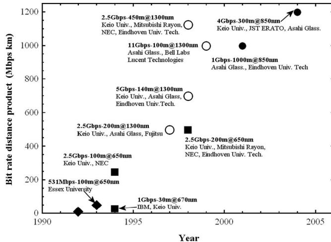
Fig. 2. Development of data rate achieved by POF links. ■ GI POF at 650 nm. ● GI POF at 850 nm. ○ GI POF at 1300 nm. ◆ SI POF.
