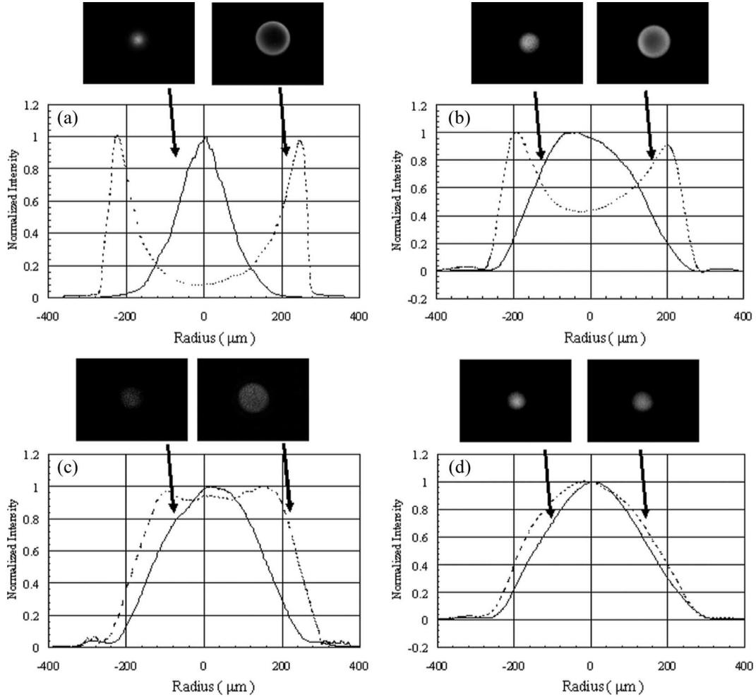
Fig. 4. Fiber NA dependence of NFPs of 100-m GI POF (NA: 0.15–0.30). Two-dimensional photos and normalized power distribution in radial direction. Solid line: center launch. Broken line: Peripheral launch (offset). (a) NA = 0.30. (b) NA = 0.20. (c) NA = 0.17. (d) Fiber 2 NA = 0.15.
