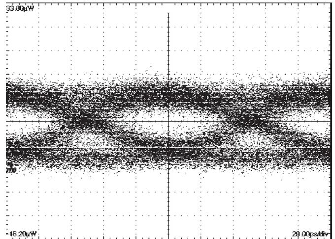
Fig. 17. Eye diagram of 10 Gb/s data transmission after a 100-m PF GI POF with ideal index profile at 850-nm wavelength.
