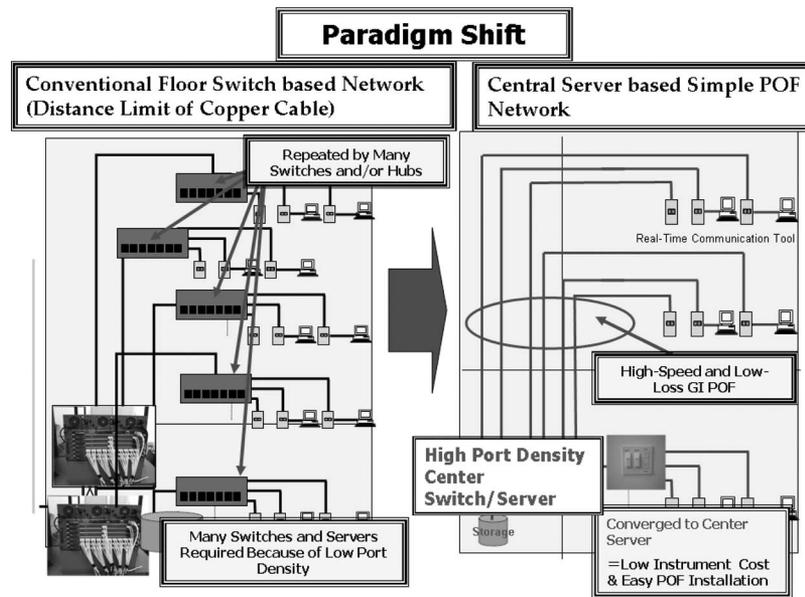
Fig. 19. Concept of centralized network architecture realized with high-bandwidth GI POF.
