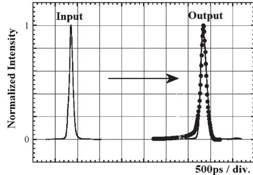
Fig. 7. Pulse broadening through 150-m fiber. Closed circle: estimated output waveform from the measured index profile. -3-dB bandwidth: 2.88 GHz.
