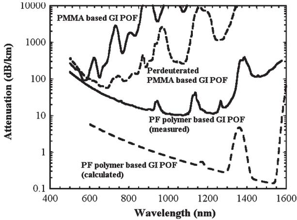
Fig. 11. Attenuation spectra of GI POFs.
