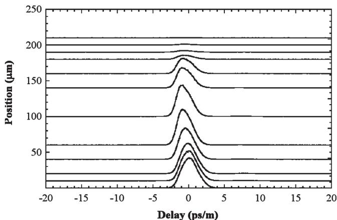
Fig. 8. DMD measurement results of 100-m fiber.
