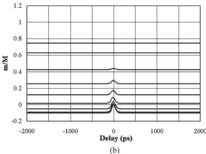
Fig. 14. DMD measurement results of 100-m PF GI POF at 650-nm wavelength. Vertical axis ( $m/M$ ) is the normalized principal mode number;  $m$  is the principal mode number, and  $M$  is the maximum principal mode number. (a) PF GI POF prepared by the conventional process. (b) PF GI POF prepared by the interfacial-gel polymerization process.
