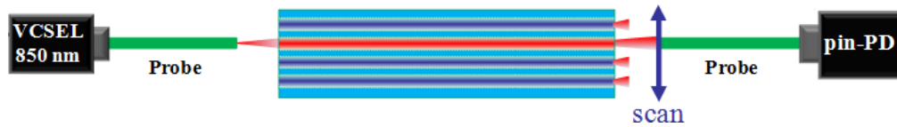
Fig. 6. Experiment setup for inter-channel crosstalk measurement.
