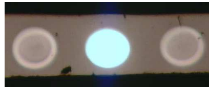
Fig. 3. The middle core of 1-m long copolymer based waveguide was launched for crosstalk measurement. We can observe the ring like pattern in adjacent channels. In this sample, the core radius of each core is approximately 50 \mu\text{m} and pitch (from the center to center) is approximately 200 \mu\text{m} .
