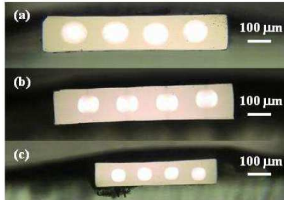
Fig. 3. Cross sections of the 4-channel GI type waveguide with (a) circular cores, (b) 100 x 100 \mu\text{m} rectangular cores and (c) 60 x 60 \mu\text{m} rectangular cores
