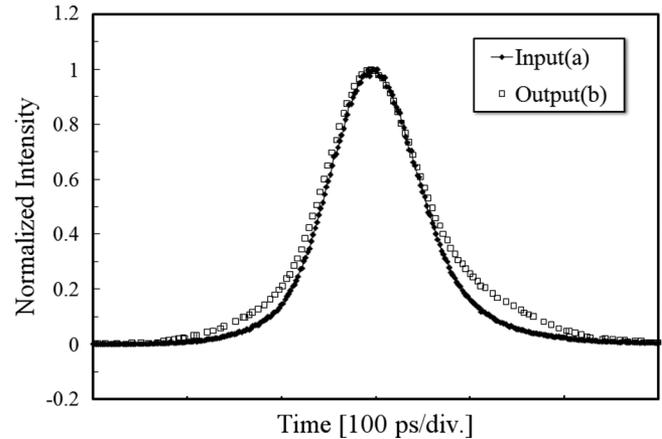
Fig. 4. Waveforms of input pulse ( $\bullet$ ) and output pulse ( $\square$ ) after a 5.0-m waveguide transmission at a wavelength of 850 nm.
