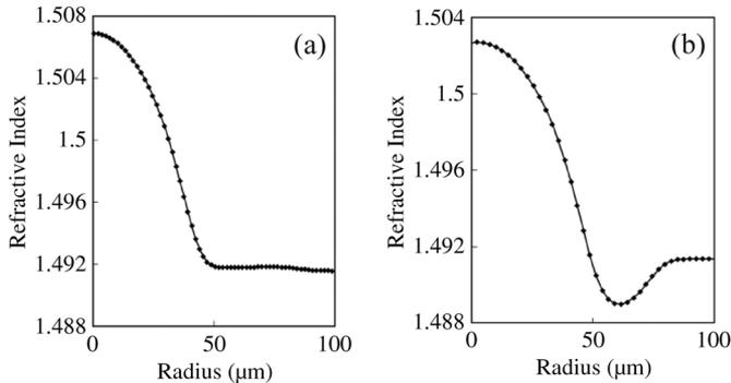
Fig. 2. Refractive index profile of a core of the waveguide with (a) GI profile and (b) W-shaped index profile.
