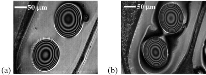
Fig. 1. (a) Interference fringe pattern of 100- $\mu\text{m}$  core waveguide with GI profile. (b) Interference fringe pattern of 100- $\mu\text{m}$  core waveguide with W-shaped profile.
