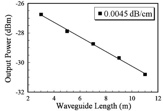
Fig. 3. Cutback plot of one channel of the waveguide (B).
