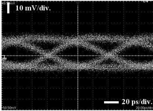
Fig. 5. Eye diagram at 12.5 Gb/s after propagation through a 15-m waveguide (100- $\mu\text{m}$  diameter core) at 850-nm wavelength.
