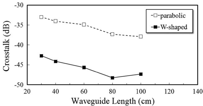
Fig. 6. Crosstalk at various lengths of two waveguides. The plot ( $\square$ ) represents acrylate-based GI waveguide, and the plot ( $\blacksquare$ ) represents perdeuterated acrylate-based W-shaped waveguide.
