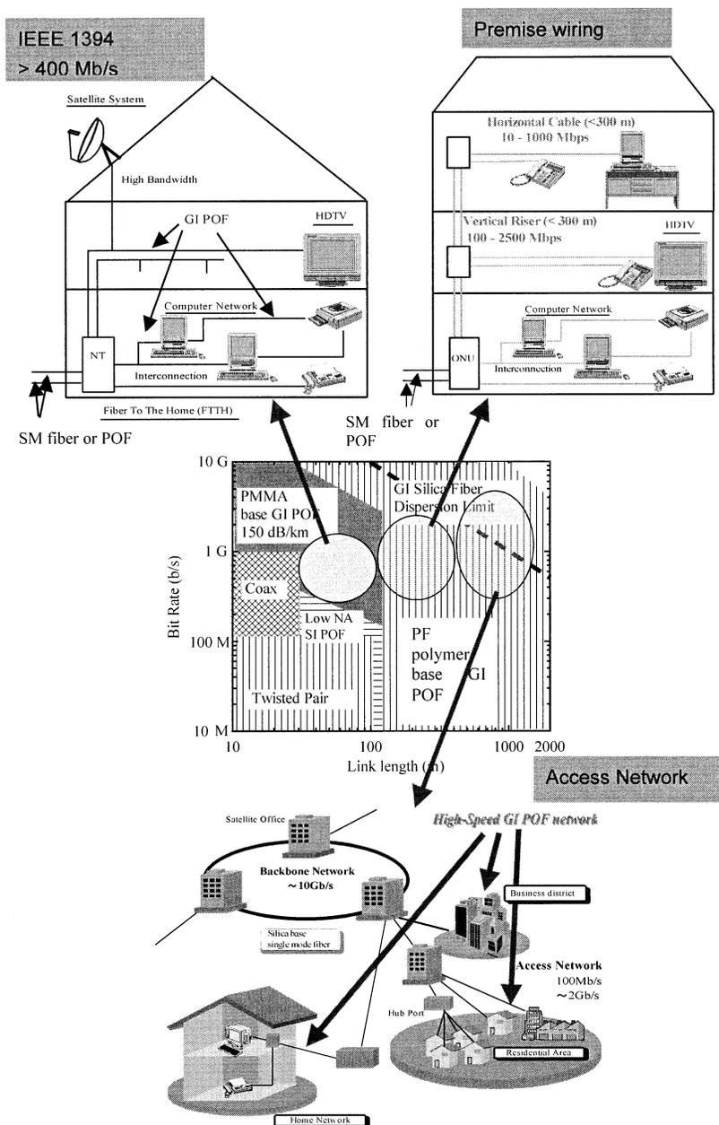
Fig. 13 Relation between the bit rate and link length of POF.
