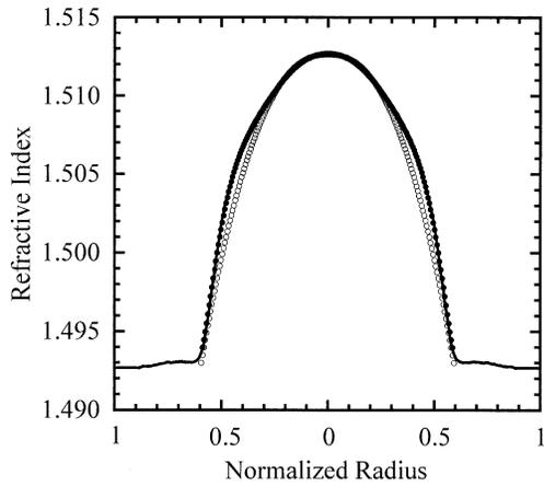
**Fig. 9** Refractive index profile of the PMMA base GI POF. Solid Line: Experimentally measured data,  $\circ$ : approximated index profile by power-law equation,  $\square$ : approximated index profile by polynomial equation.
