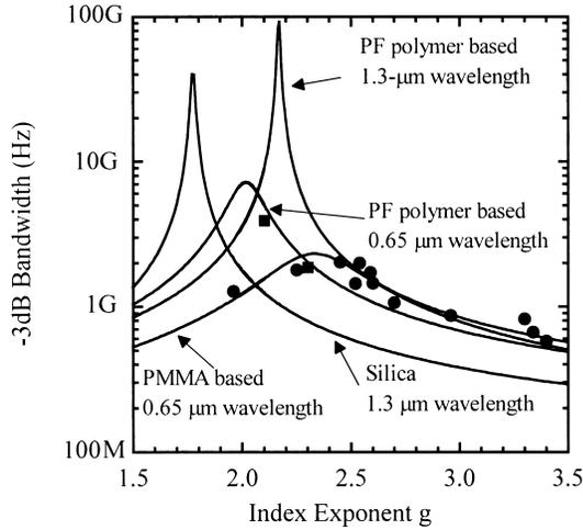
**Fig. 6** Relation between the refractive index profile and bandwidth of 100 m GI POF.  $\circ$ : Experimental data of PMMA polymer base GI POF at  $0.65 \mu\text{m}$ ,  $\blacksquare$ : Experimental data of PF polymer base GI POF at  $0.65 \mu\text{m}$ .
