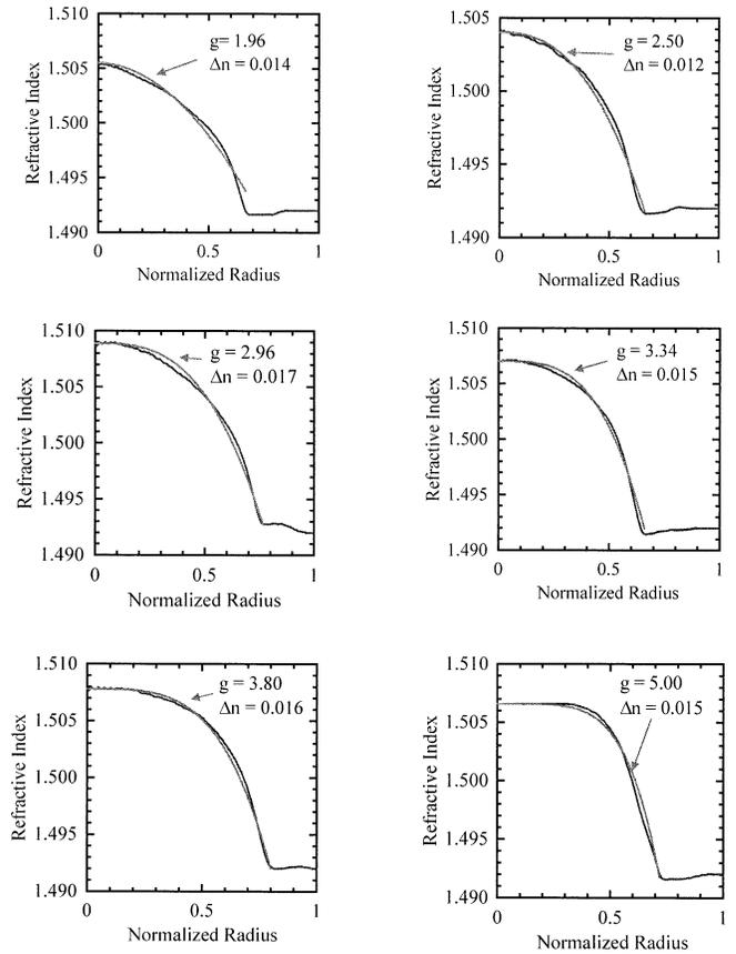
**Fig. 7** Refractive index profile of GI POFs controlled in the interfacial gel polymerization process.
