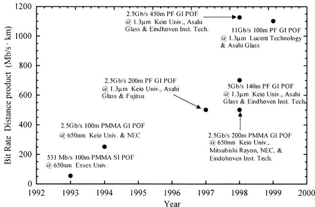
Fig. 4 Development in the high-bit rate trial in the POF link.
