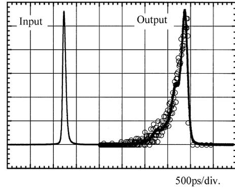
**Fig. 10** Pulse broadening through 100-m PF polymer base GI POF whose index profile is shown in Fig. 8. Signal wavelength is  $0.65 \mu\text{m}$ . Solid Line: Experimentally measured data,  $\circ$ : calculated output waveform in which uniform launch condition was taken into account.
