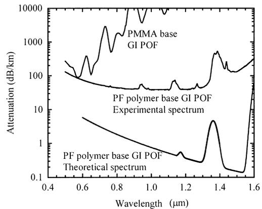
**Fig. 3** Total attenuation spectra of GI POF.
