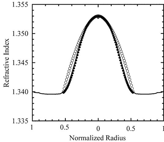
**Fig. 8** Refractive index profile of the PF polymer base GI POF. Solid Line: Experimentally measured data,  $\circ$ : approximated index profile by power-law equation,  $\square$ : approximated index profile by polynomial equation.
