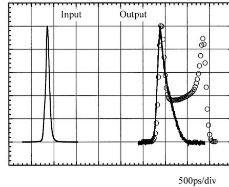
**Fig. 11** Pulse broadening through 100-m PMMA base GI POF whose index profile is shown in Fig. 9. Signal wavelength is  $0.65 \mu\text{m}$ . Solid Line: Experimentally measured data,  $\circ$ : calculated output waveform in which uniform launch condition was taken into account.
