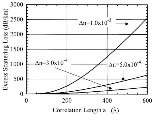
**Fig. 2** Excess scattering loss due to heterogeneous structure in polymers.
