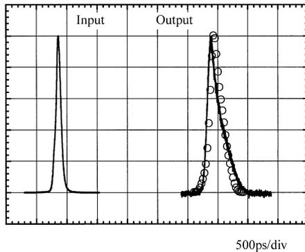
**Fig. 12** Pulse broadening through 100-m PMMA base GI POF whose index profile is shown in Fig.9. Signal wavelength is  $0.65\ \mu\text{m}$ . Solid Line: Experimentally measured data,  $\circ$ : calculated output waveform in which mode dependent attenuation was taken into account.
