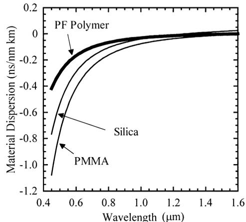
Fig. 5 Material dispersion of polymers compared with silica.
