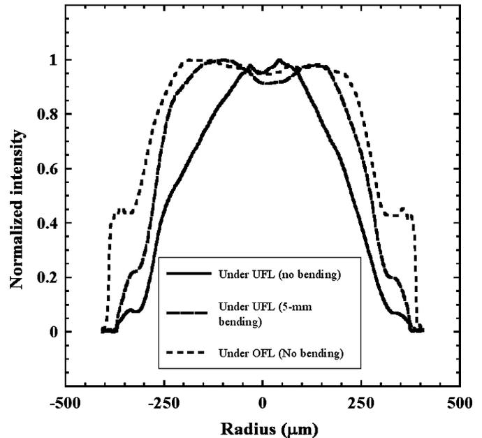
Fig. 10. Output near field patterns (NFPs) of the PVDF-clad GI POF under the RML condition before and after static fiber bending.
