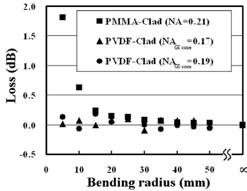
Fig. 8. Comparison of bending losses between the PVDF-clad GI POF and the conventional PMMA-clad GI POF.
