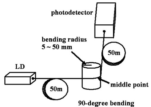
Fig. 3. Schematic representation of the measurement condition of bending loss of GI POF.
