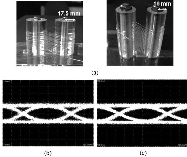
Fig. 11. (a) Photo of the bending condition of the PVDF-clad GI POFs and eye patterns after a 1.25 Gb/s data transmission by the PVDF-clad GI POFs with static fiber bendings. (b) Bending radius = 17.5 mm. (c) Bending radius = 10 mm.
