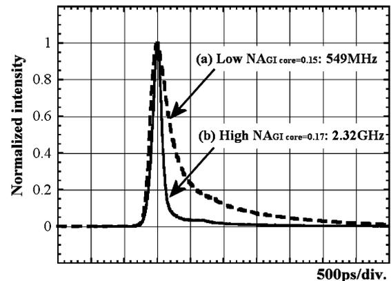
Fig. 7. Output pulse waveforms from the 100-m PVDF-clad GI POFs with different NA in their GI core regions when they are launched under the RML condition.
