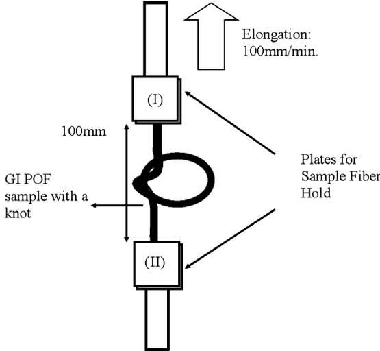
Fig. 2. Schematic representation of the measurement condition of knot tensile strength.
