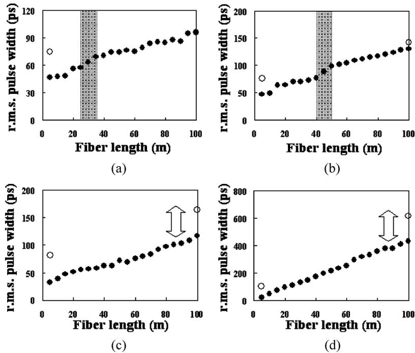
Fig. 5. Relationship between output pulse width and fiber length from GI POFs with different NA. Closed circle: Measured under the RML condition. Open circle: Measured under the OML condition. (a) Fiber A NA = 0.14. (b) Fiber B NA = 0.17. (c) Fiber C NA = 0.19. (d) Fiber D NA = 0.22.
