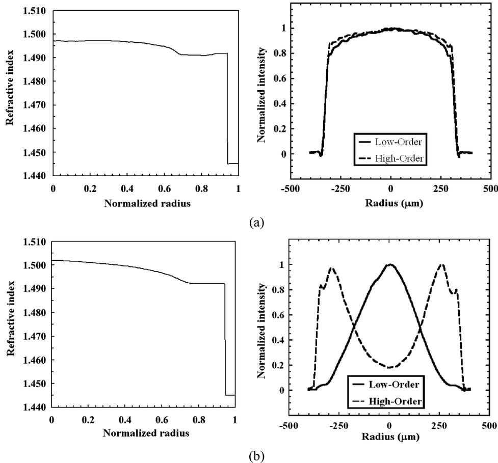
Fig. 6. Refractive index profile of PVDF clad GI POFs with different NA and their output near field patterns (NFP) of low-order and high-order mode groups launched separately. (a) Fiber E  $NA_{GI\ core} = 0.15$ . (b) Fiber F  $NA_{GI\ core} = 0.17$ .
