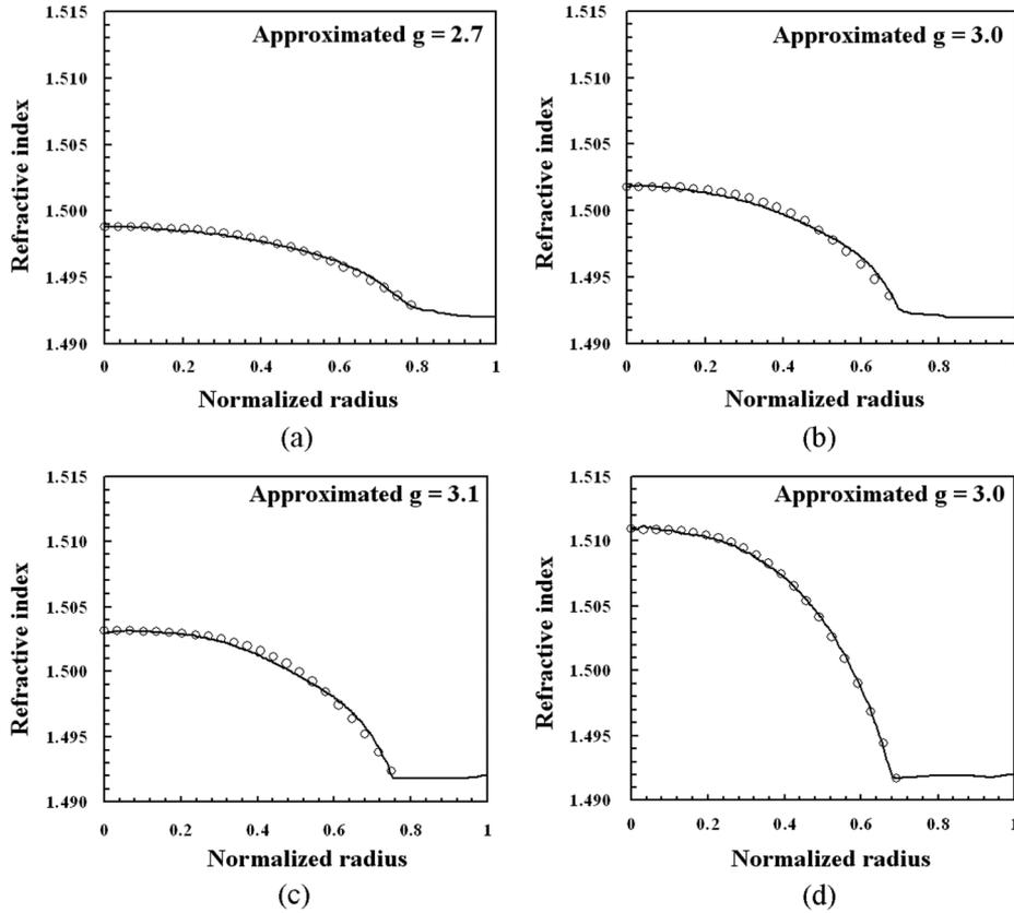
Fig. 4. Refractive index profiles of the PMMA-clad GI POFs with different NA. Solid line: Measured index profile. Open circle: Approximated curve by power law form. (a) Fiber A NA = 0.14. (b) Fiber B NA = 0.17. (c) Fiber C NA = 0.19. (d) Fiber D NA = 0.22.
