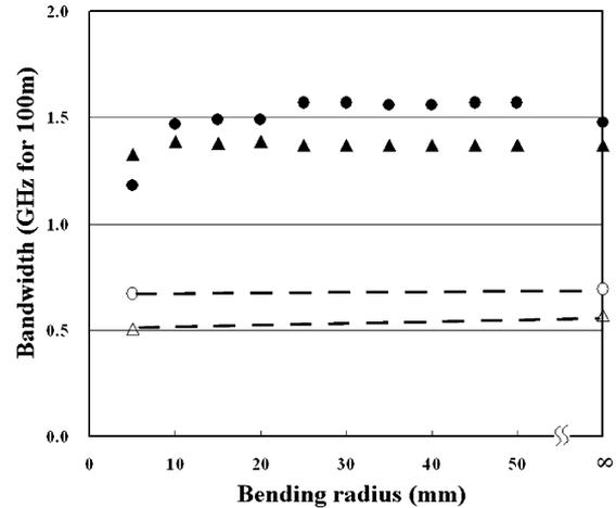
Fig. 9. Bandwidth stability of the PVDF-clad GI POFs with different NA in their GI core region. Closed circle:  $NA_{GI\ core} = 0.19$  under RML closed triangle:  $NA_{GI\ core} = 0.17$  under RML open circle:  $NA_{GI\ core} = 0.19$  under OML open triangle:  $NA_{GI\ core} = 0.17$  under OML.
