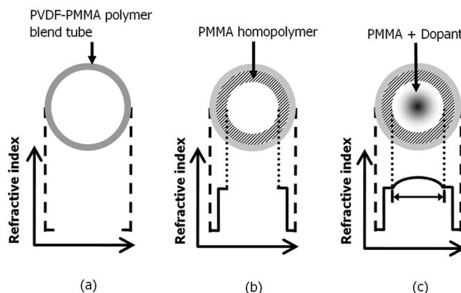
Fig. 1. Formation process of PVDF-clad GI preform rod by the Interfacial-gel polymerization technique. (a) Clad region. (b) Flat refractive index region. (c) GI core region.
